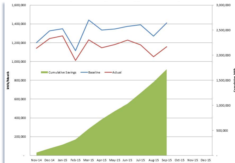
Figure 4: Summary of Compressed Air System Energy Use and Savings This chart shows the clear reduction in energy usage by the Compressed Air System following the modifications made during this project (red line). It highlights the dramatic cumulative savings provided by Monitoring-based Commissioning
