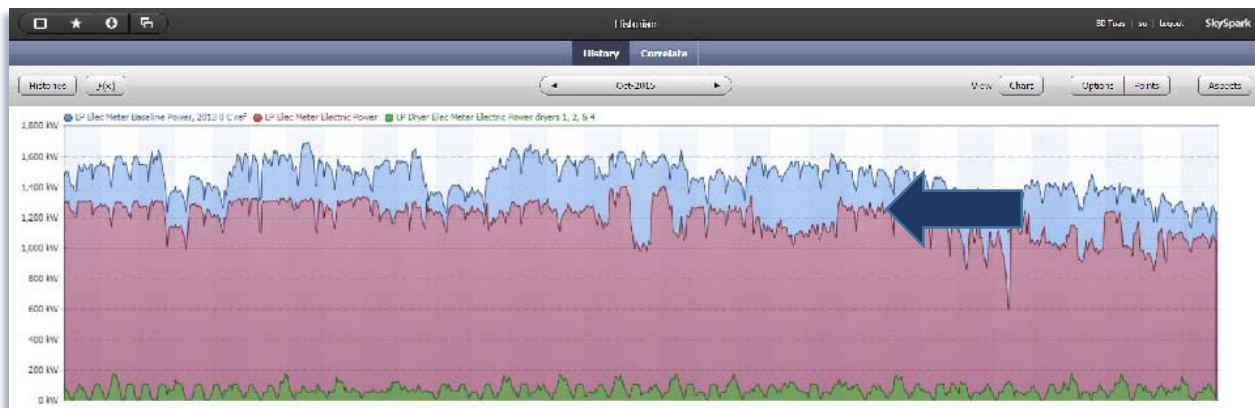
Figure 2: Baseline vs. Actual Energy Use The difference in baseline power calculated (blue) compared to actual power (red) demonstrates savings over time due to implementation of efficiency measures.
