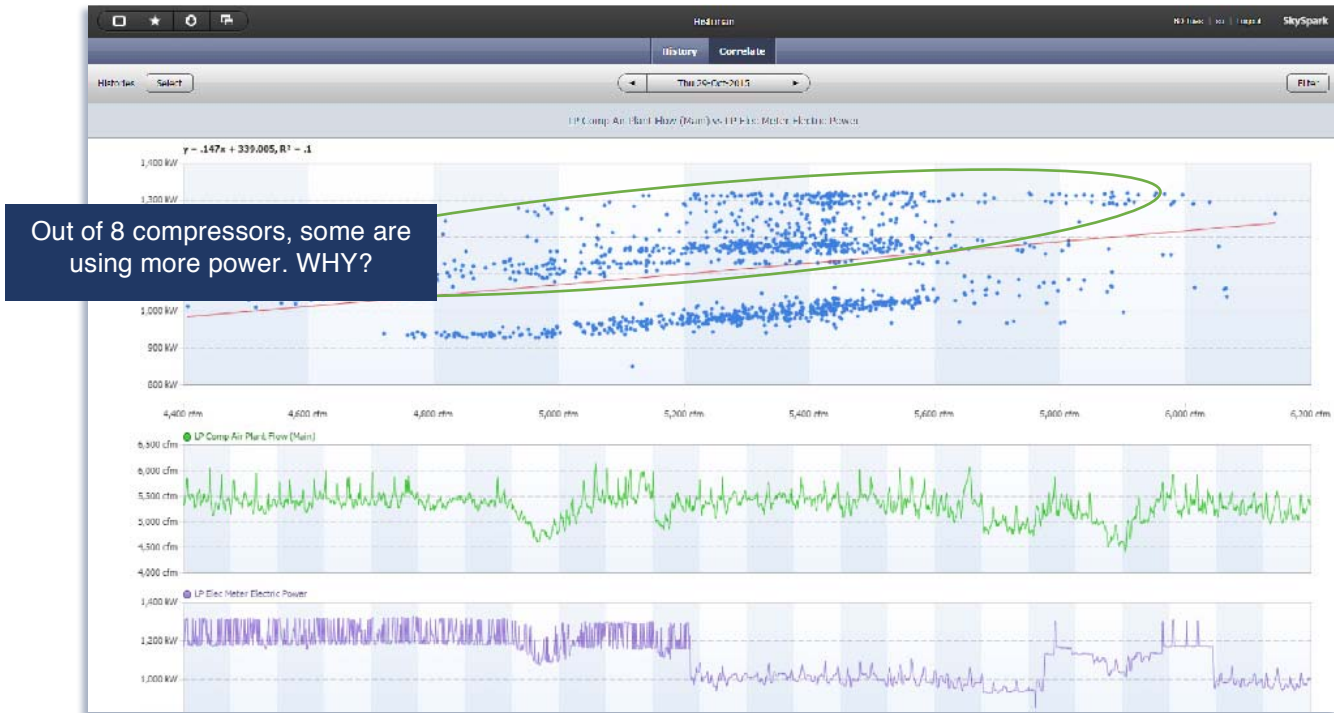
Figure 1: Power and Flow Correlation – Operational Insight Note the large fluctuations in power, while flow and pressure remain relatively constant. We worked with plant operators to evaluate compressor staging.
